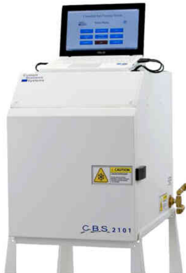
Figure 7.3.1: The CBS CRF2101 controlled-rate freezer. The CRF2101 uses liquid nitrogen to provide for the controlled-rate freezing of biological samples, with freezing data being collected according to 21 CFR Part 11 requirements by the onboard laptop controller.
